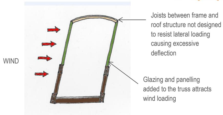
Fig. 5 Truss enclosed with glazing and roof
