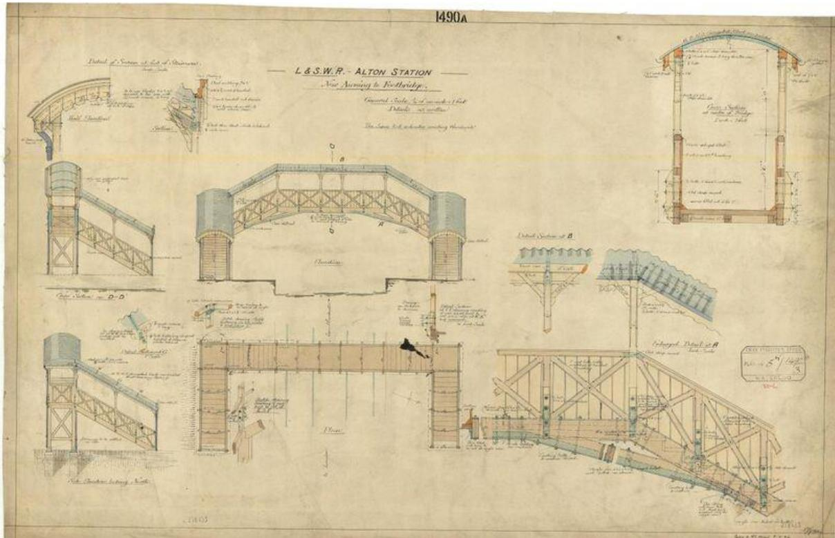
Figure 1 – LSWR drawing of planned cladding and roof at Alton.
