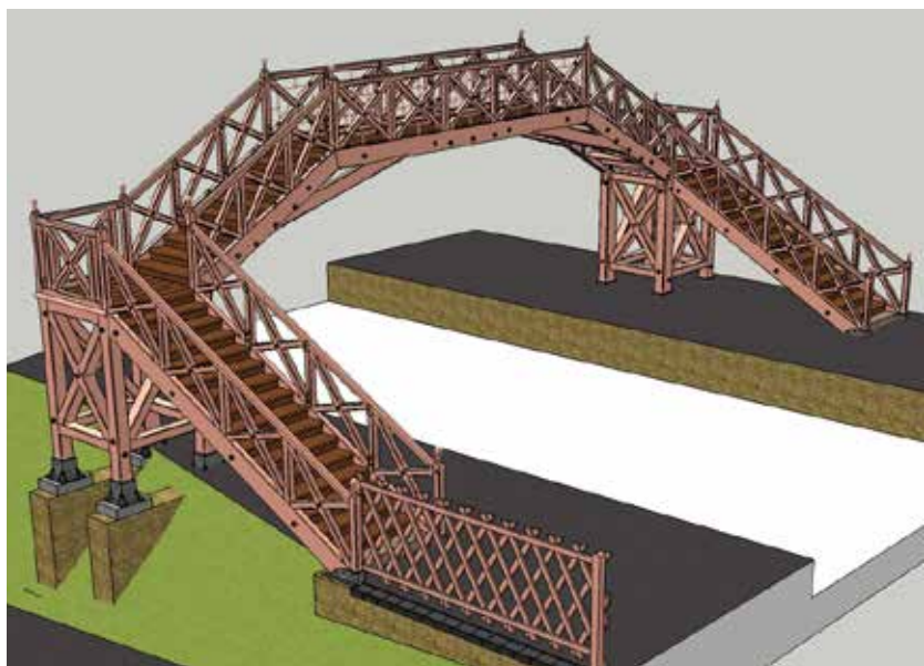
Alton's footbridge recreated in 3D CAD, using the original LSWR plans as the basis. In practice, it was built as per Wadebridge.
